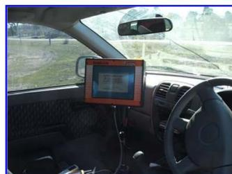
RTK GPS Mounted in a 4WD Vehicle
