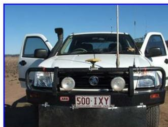
RTK GPS Mounted in a 4WD Vehicle
